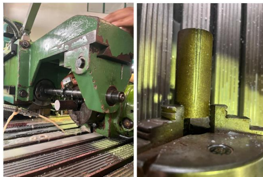
Fig. 4. Measurement process with cutter diameter 55.25 mm
