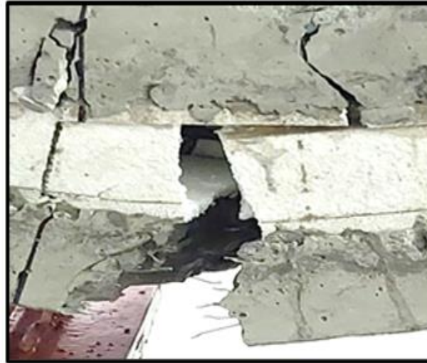
Fig. 12. Steel fiber holding the upper layer
