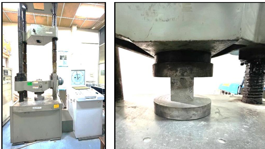
Fig. 5. Set up for testing compressive strength of foamed concrete after 28 days
