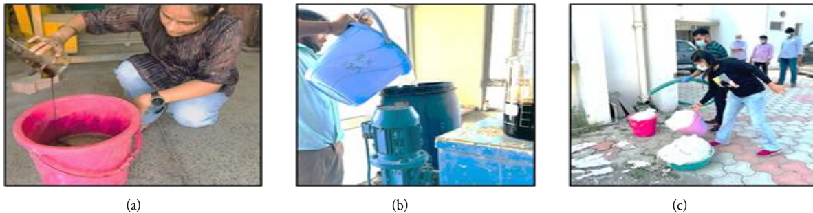
Fig. 2. (a) Dilution of foaming agent, (b) Set up of foam generator, and (c) Collection of foam
