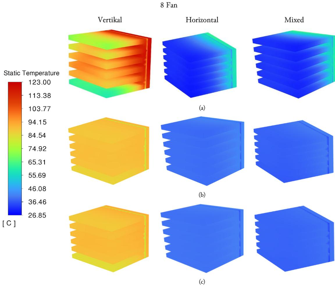
**Fig. 6.** Static temperature contours of Processor and Heat Sink (a) Steel, (b) Aluminum, (c) Copper
