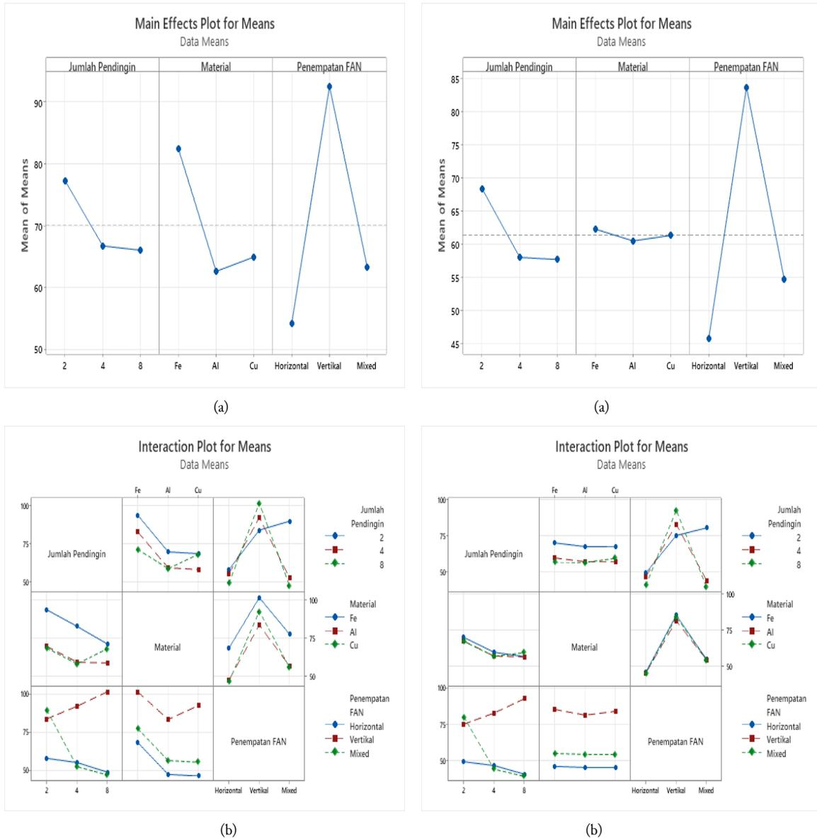
Fig. 4. Main effect plot for means processor temperature response (a), sink temperature response(b)
