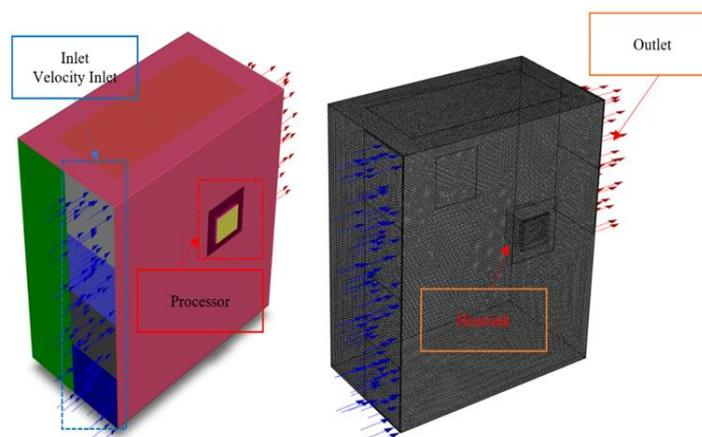
Fig. 2. CPU casing model, Boundary Condition, and Mesh
