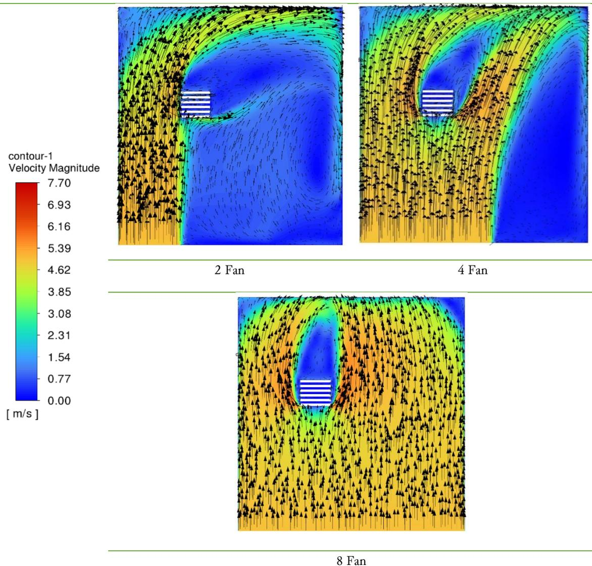
**Fig. 8.** Velocity Contour with vector velocity on vertical configuration (a) 2 Fan, (b) 4 Fan, and (c) 8 Fan
