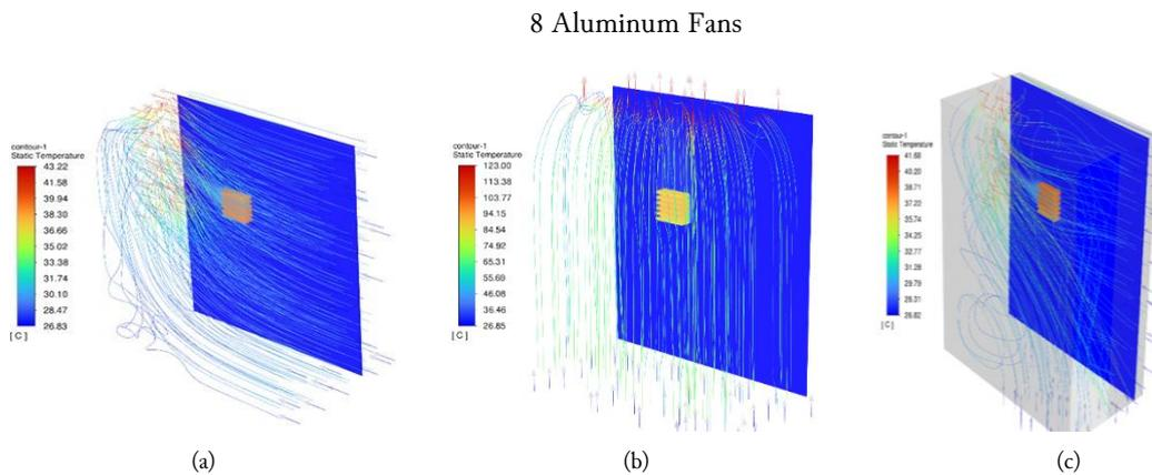
**Fig. 7.** Temperature Contour with Pathline Velocity on 8 Aluminum Fan design variations (a) Horizontal, (b) Vertical, (c) Mixture
