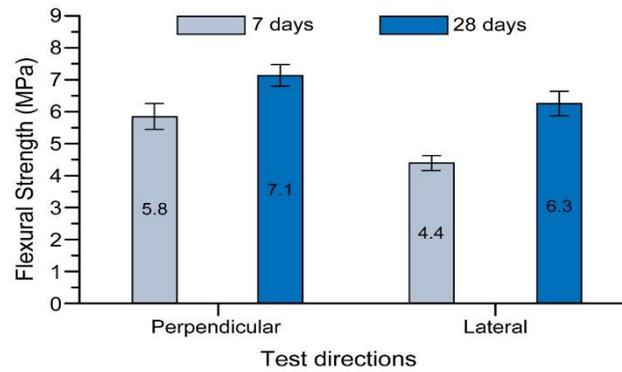
Fig. 8. Tensile Strength in Different Orientations Obtained from Optimum Mixture for 3D Printing [28]
