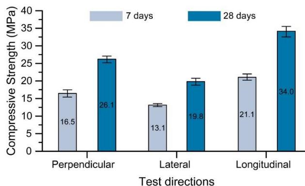
**Fig. 7.** Compression strength in different orientations obtained from the optimal blend for 3D printing [28]
