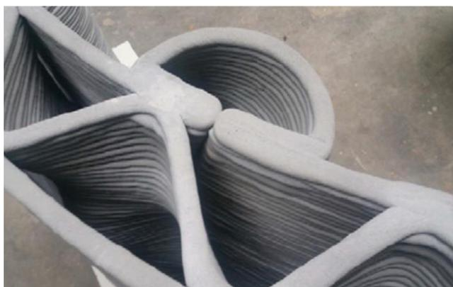
Fig. 12. Layered Appearance of a 3D Printed Concrete Structure [54]
