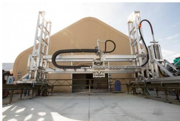
Fig. 5. The Schematic of An Automatic CC System [57]
