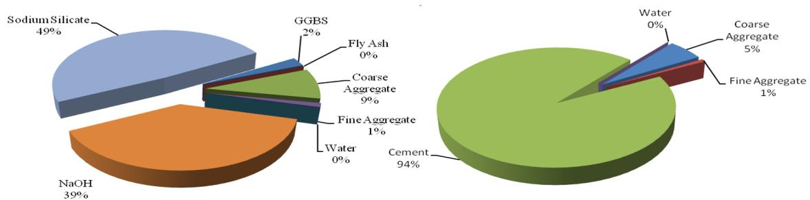
**Fig. 6.** Energy share of individual materials. Left: Fly ash GP concrete; Right: OPC concrete [100]
