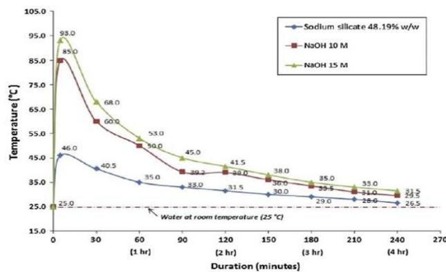
Fig. 11. The Effect of Alkaline Solution on Initial Curing Temperature [121]
