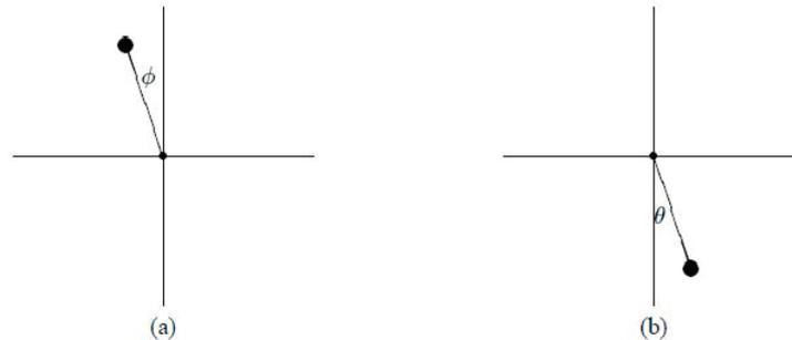
**Fig. 1.** Local models of the pendulum (where  $\phi = \theta - pi$ ): (a)  $\phi = 0$  at the unstable fixed-point, and (b)  $\phi = 0$  at the stable fixed-point.
