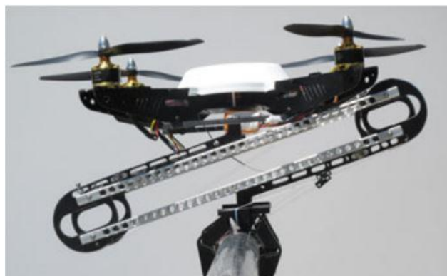
Fig. 5 Quadrotor perching on a cylindrical railing. The grip is actuated by the weight of the quadrotor [16].
