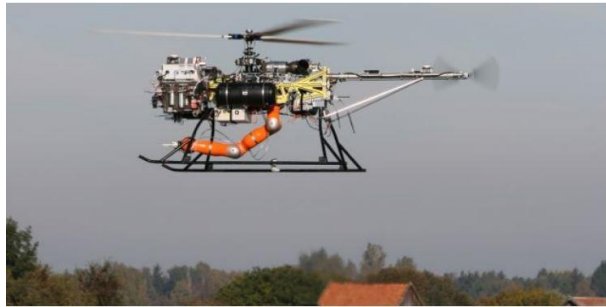
Fig. 4. First experimental platform for aerial manipulation with a 7DoF industrial manipulator based on a main-tail-rotor helicopter [13].
