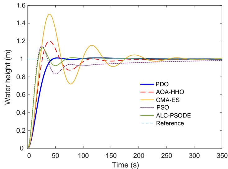
Fig. 5. Step response of different optimizers-based controller designs for water height
