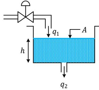
Fig. 2. Simplified structure of a tank
