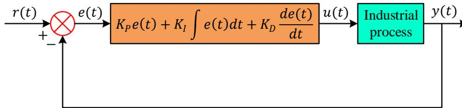
Fig. 1. Block diagram of a PID controlled three-tank system for industrial processes
