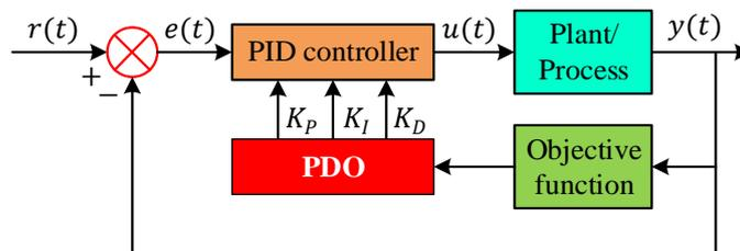
Fig. 3. Implementation procedure showing the minimization with PDO and  $F$  objective function
