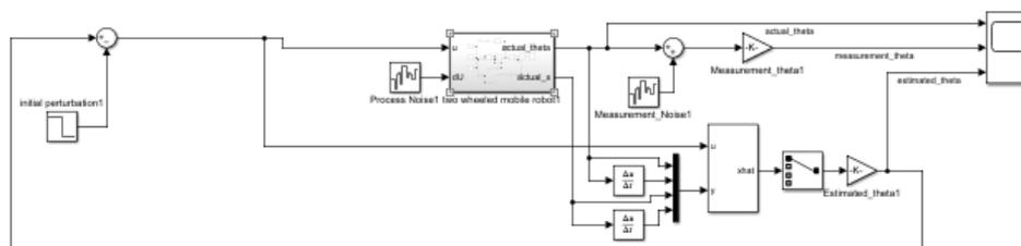
Fig. 7. Control simulation of two-wheeled mobile robot using Kalman Filter
