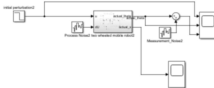
Fig. 5. Block diagram without control
