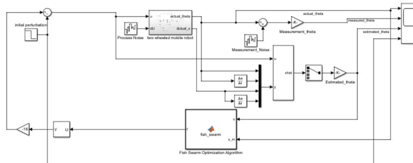
Fig. 9. Control simulation of two-wheeled mobile robot using kalman Filter-FSOA
