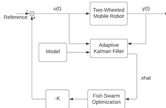
**Fig. 1.** Block diagram stabilizing mobile robot using Kalman Filter and fish swarm optimization algorithm
